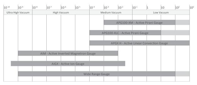
The dark grey shading indicates the primary accuracy range for the specified gauge.
